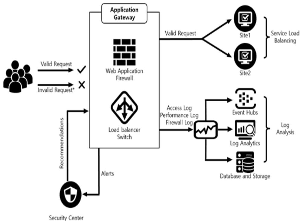
Invalid requests are usually blocked as soon as they are detected, while valid traffic (Valid Requests) is appropriately distributed and managed on internal web servers to serve users. In the event of an issue with ClebusX's control system (Application Gateway), the Security Center suggests issues for checking. Once the suggestions are delivered, internal security experts analyze the logs loaded into the control system and track events to detect security issues and respond according to policy.
