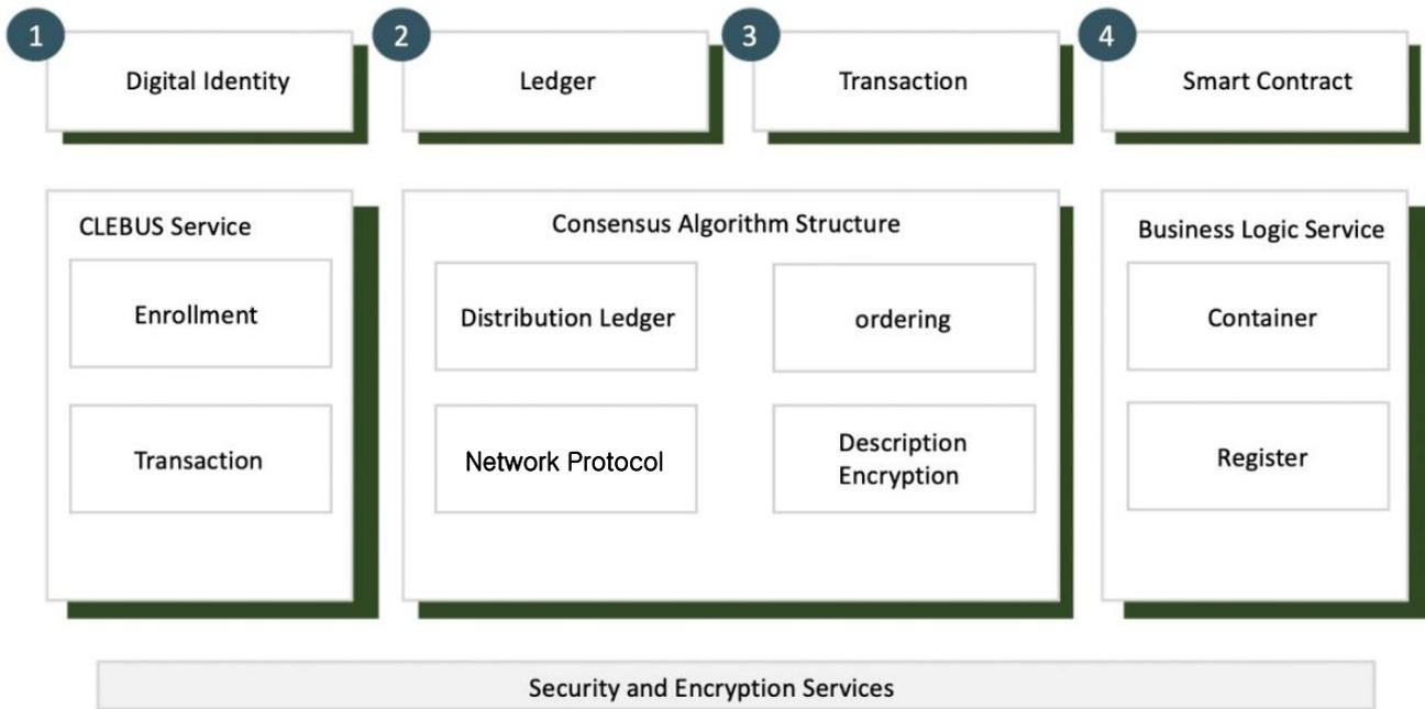
① Identity verification layer for securing CLEBUS data. DID authentication of users is mandatory for transactions in CLEBUS. Participants store relevant data in the distributed ledger for recording, modifying, and deleting, and provide functions for issuing related certificates.
